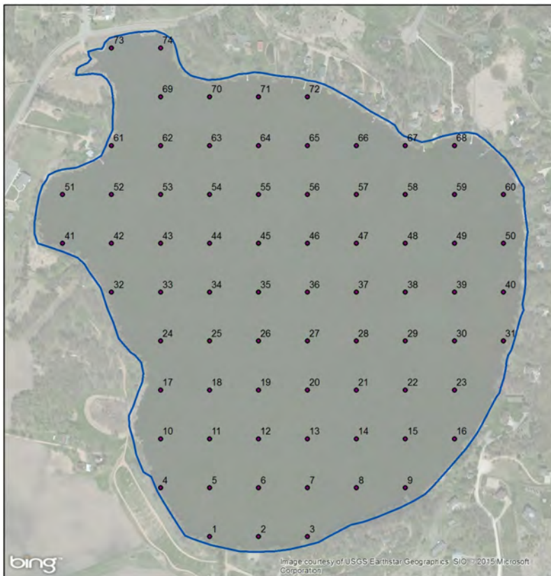
Figure 1. Point intercept sample sites for Fish Lake in 2022. Sample sites were spaced 100 meters apart.
