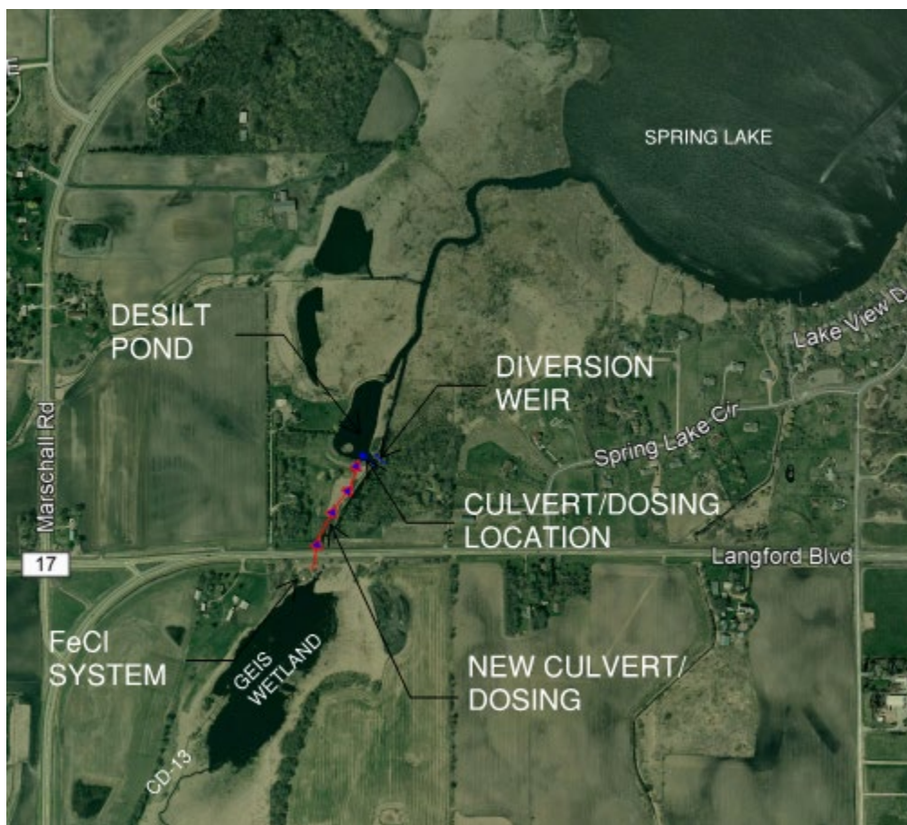
Figure 5.10. Ferric Chloride System improvements alternative 1.
