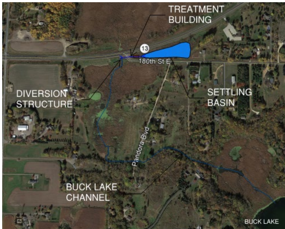
Figure 5.13. Buck Lake chemical treatment system.
