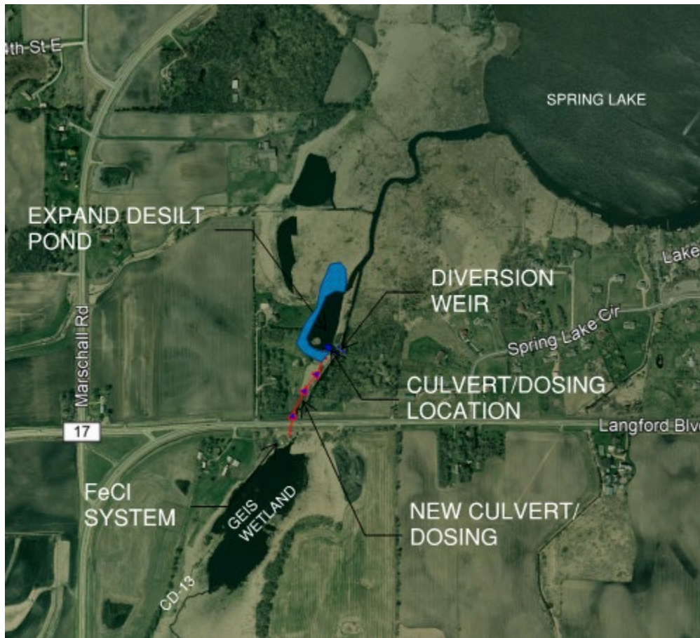
Figure 5.11 Ferric Chloride system improvements alternative 2
