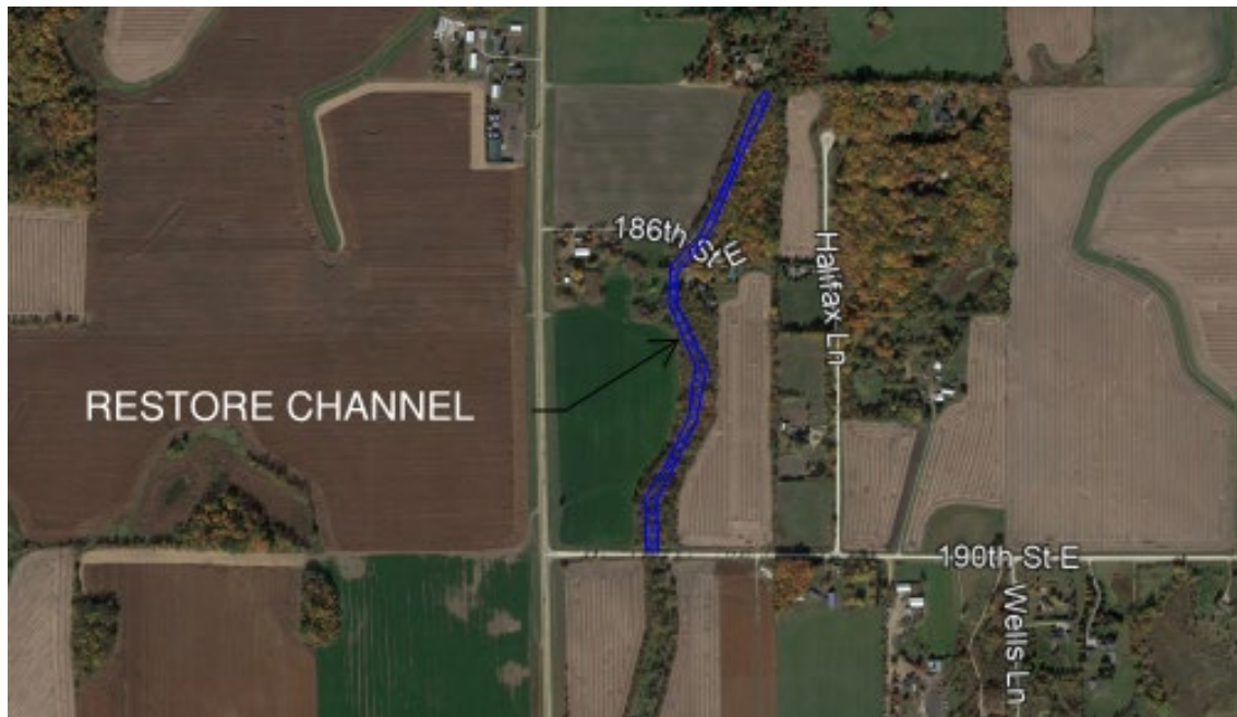
Figure 5.8. County Ditch 13 repairs south of Geis Wetland.
