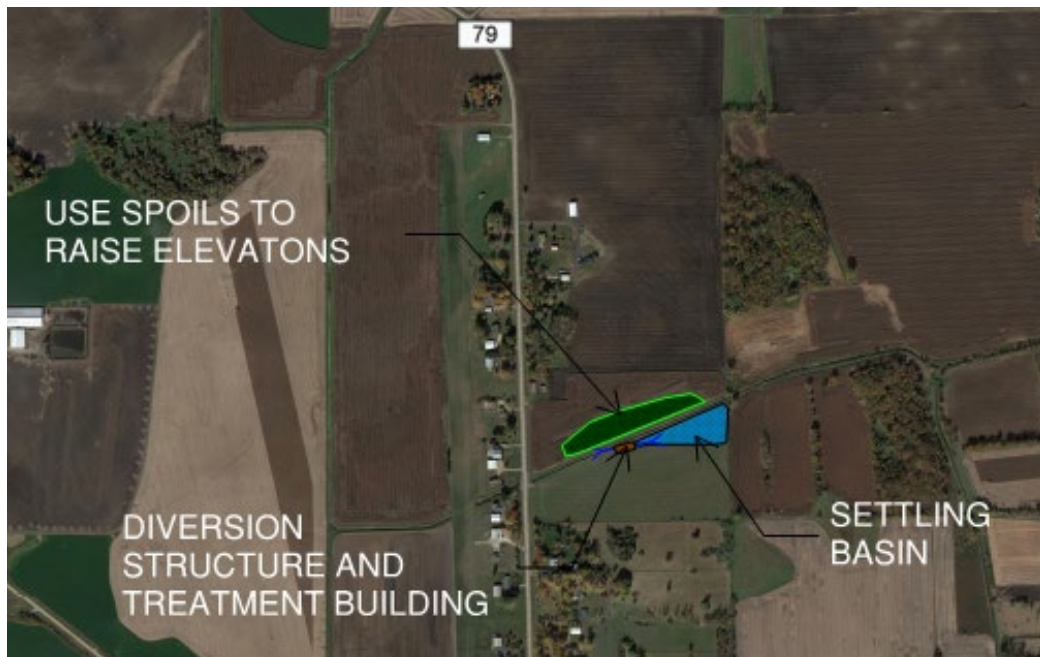
Figure 5.14. County Ditch 13 chemical treatment system.
