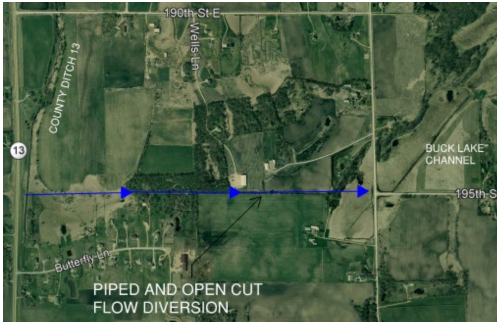
Figure 5.9. County Ditch 13 Diversion.
